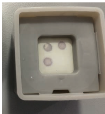
Figure 4. A Multispot test positive for HIV 1 The first spot on the left represents positive control and two spots on the right indicate positive HIV 1 disease.
